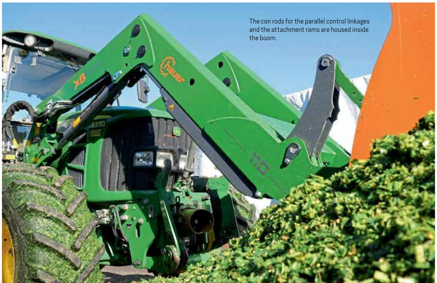
The con rods for the parallel control linkages and the attachment rams are housed inside the boom.
