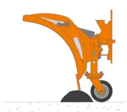
Return springs maintain the snow blade in its working position and yet allow the blade to float over small obstacles by moving up and only a few centimetres to the rear.
