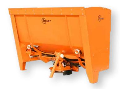
Whit the new construction of the TS-3 the main emphasis was put on a process and function based design. The new spreader now offers new features and is ideal for spreading material on streets, roads and parking lots. Developed with a focus on close attachment to the three-point linkage for optimum weight distribution, the implement offers the best possible ride on snow and ice covered surfaces.
